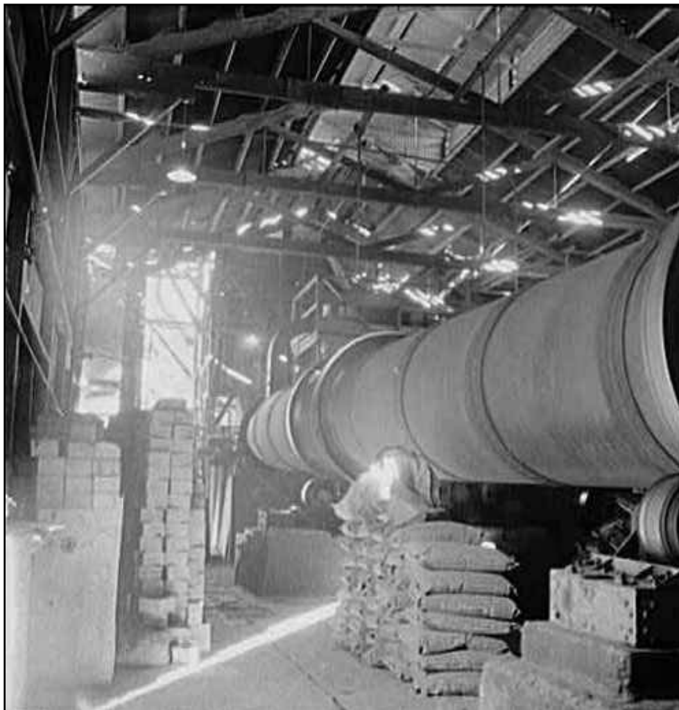
Figure 3.13-7: Gould Rotary Furnace at New Idria 1942 (A. Feininger, Office of War Information, National Archives).
